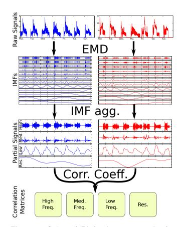
Figure 3: Strip and Bind using two raw signals standing for one week of data from two different HVACs. (1) Decomposition of the signals in IMFs using EMD (top to bottom:  $c_1$  to  $c_n$ ); (2) aggregation of the IMFs based on their time scale; (3) comparison of the partial signals (aggregated IMFs) using correlation coefficient.
