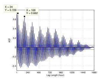
Figure 2: Auto-correlation of a usual signal from the Building 1 dataset. The signal features daily and weekly patterns (resp. x = 24 and x = 168).
