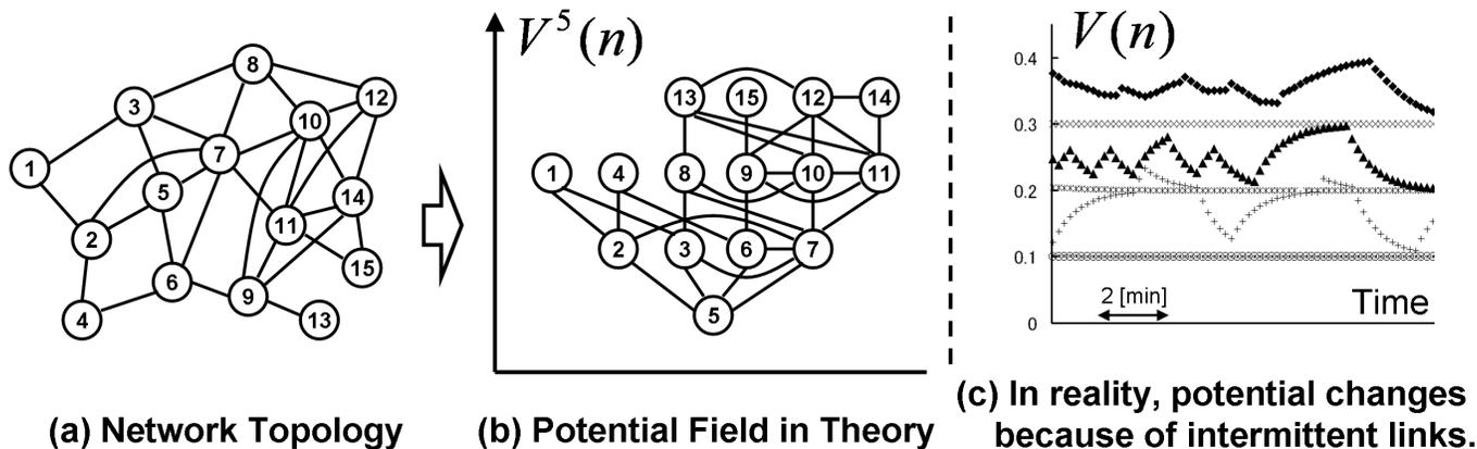
Fig. 6. Potential field construction (in theory and in reality); potential-field converges into (b) if the given network topology (a) does not change. However, links are intermittent and the topology dynamically changes. Potential-field follows this change as (c). (c) is a real trace on UTMesh.
