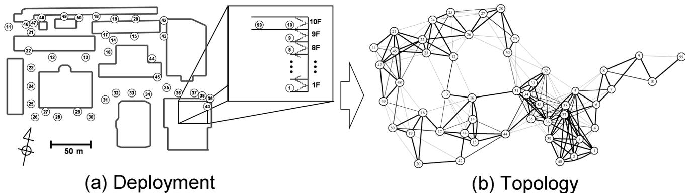
Fig. 2. (a) The experiment setting to analyze intermittent links between wireless nodes deployed in ad hoc manner. (b) Summarized network topology; bolder link indicates higher link availability.
