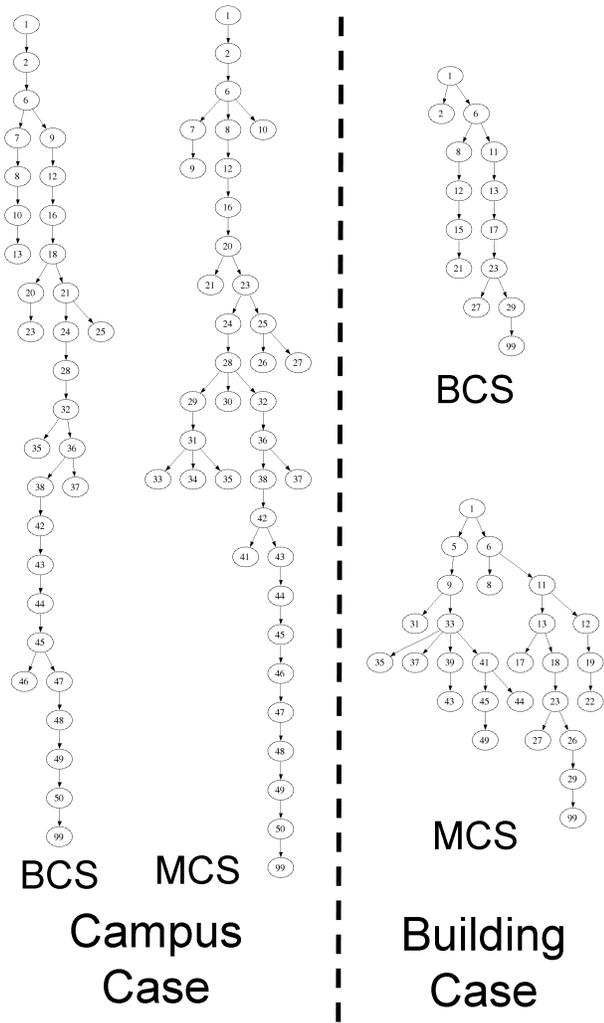
Fig. 10. Message delivery pattern examples from source 1 to destination 99. PEAR achieved scalable message propagation in hop count. MCS made larger number of replicas, found faster delivery path, and took bigger hop count than BCS.
