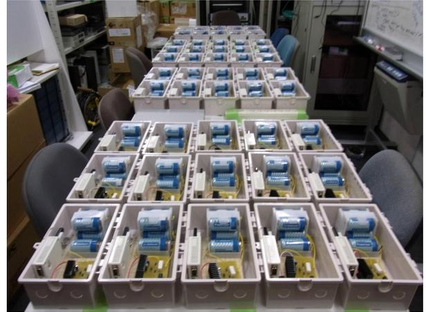
Fig. 1. UTMesh overview: 50 wireless nodes (5 lines  $\times$  10 rows) gathered at the laboratory, in Eng. Bldg. 2 at the University of Tokyo.
