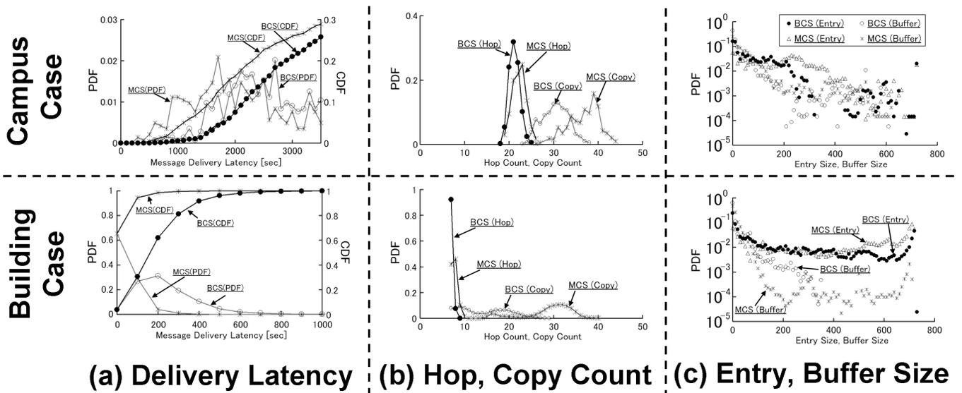
Fig. 9. The distributions of (a) delivery latency, (b) hop and copy count, (c) entry and buffer size for campus case and building case.
