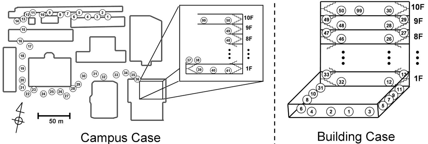
Fig. 7. Deployment configuration; we deployed 51 nodes in Hongo campus (campus case) and Eng. Bldg. 2 (building case) in the University of Tokyo.
