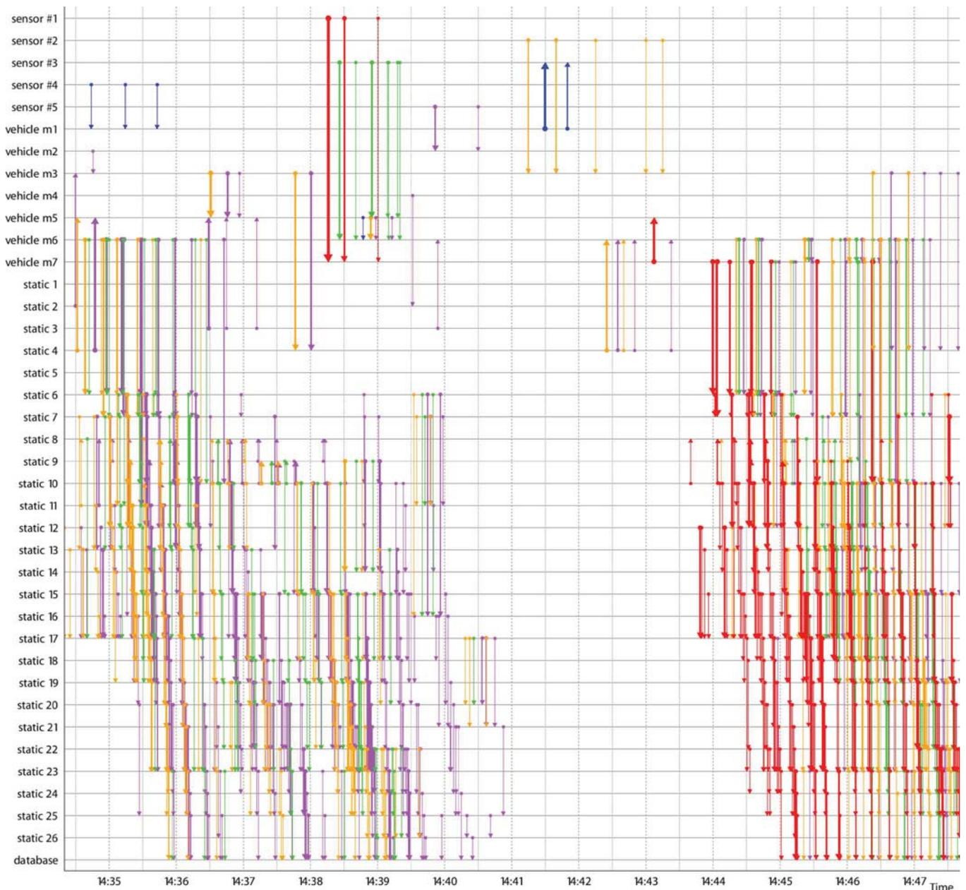
Fig. 8. Dataflow from the sensors (#1, #2, #3, #4, #5) to the database. An arrow shows data transmission between the nodes. Bolder arrows sent larger number of data at the same time. The color corresponds to the source of the data flows as (#1, #2, #3, #4, #5) = (red, yellow, green, blue, violet).
