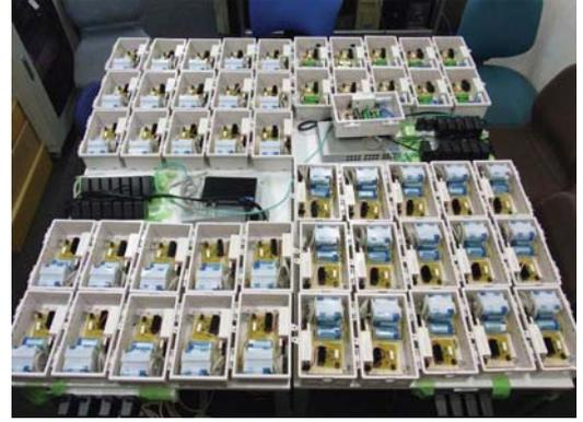
Fig. 3. DTN nodes (UTMesh) for the experiment. We configured five nodes for sensors and one node for database, used seven nodes as vehicular nodes and deployed 26 static nodes (Fig. 5 illustrates the setting of the experiment).
