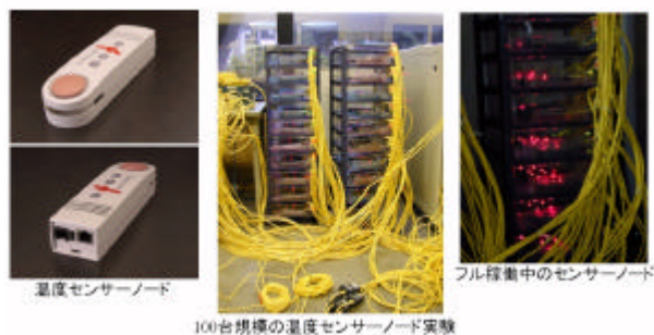
Figure 4. i-node, the first embedded sensor node in 2001
